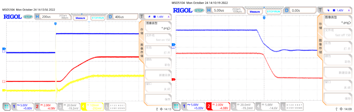
Vin slow on/off 150mA, Vout=3.3V
