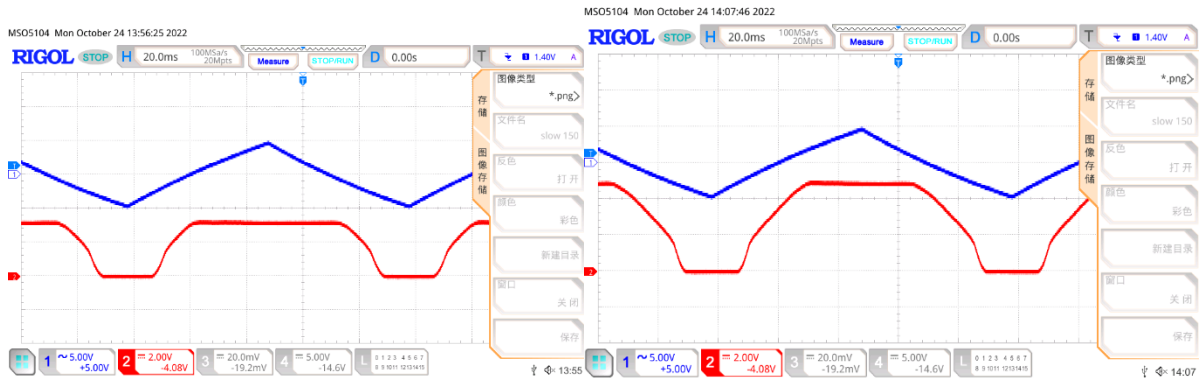
Line transient Vout=3.3V, Iout=1mA
