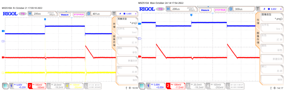
Line transient Vout=3.3V, Iout=1mA
