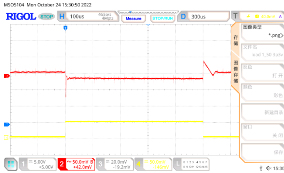
Load transient V_{out}=3.3V , I_{out}=1mA-50mA
